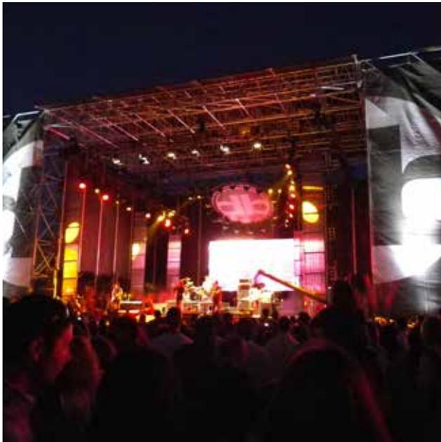
This LED Screen Ground Support in RF40 trusses and Varitower 3-30 provide high-level truss supports for flying up to 1,800 kg screens in different applications.
