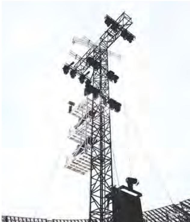
Support tower for audio systems or follow spot system. Designed in QL85A, this new Flyintower is suitable for 8,000 kg loads and can reach the height of 15,5 meters, thus ensuring sturdiness and rigidity on relevant heights. It also utilized the ballast system to stabilize itself and it creates a free area on the front to simplify the system for loading.
