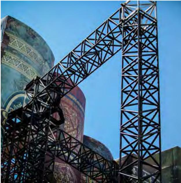
Square section High Load aluminium truss with 76 cm long sides. It is provided with steel fork connections and  $\varnothing 50 \times 4$  mm chords. Thanks to its elevated moment of inertia and resistance of its connections, it is mainly used in the composition of towers (Maxitower 76).
