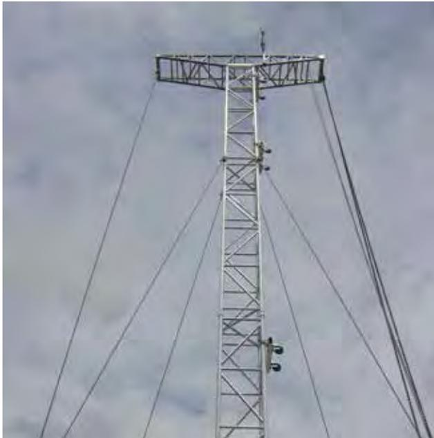
Vertical audio system support tower. It consists of QL52A structures and is suitable for lifting loads of up to 2500 kg to a height of 13 metres. The electric chain hoist is fitted directly to the top truss structure. A lifting system is available for raising the tower.
