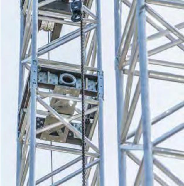
The Maxitower MT63 is the new tower for the MyT Virtue truss system. Featuring LITEC's innovative safety block with telescopic tube, it provides unrivaled levels of convenience and safety. With a maximum height of 25 metres and load capacity of 11.5 tons at 15 metres, the MT63 is the right choice for your very large and demanding projects.
