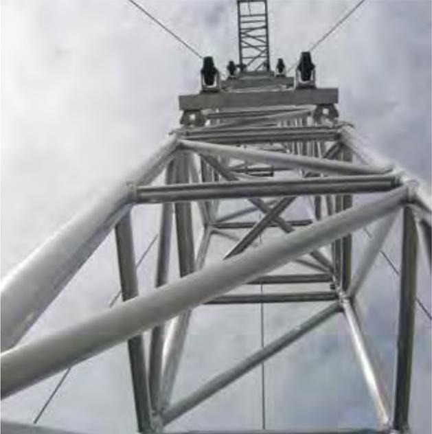
Support Tower for audio systems. Designed in QL76A, this new Flyintower is suitable for 2,000 kg loads and can reach the height of 15 meters, thus ensuring sturdiness and rigidity on relevant heights. It also utilizes QH30SA trusses as stabilizing elements and is equipped with fork connections.
