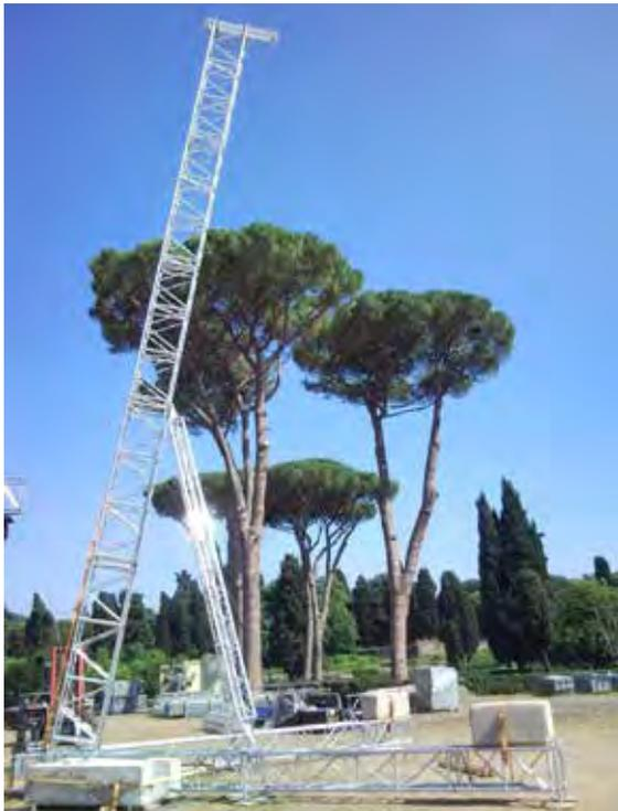
Support Tower for audio systems consisting of a QX40SA structure, suitable for lifting loads of up to 750 kg to a height of 7.5 metres or a QH40SA structure, suitable for lifting loads of up to 900 kg to a height of 9.5 metres. To lift the loads, anchoring is provided for an electric chain hoist.
